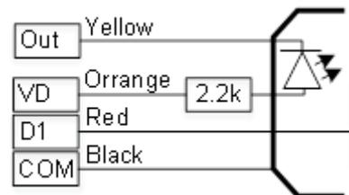
Figure 27 iButton reader wiring diagram
