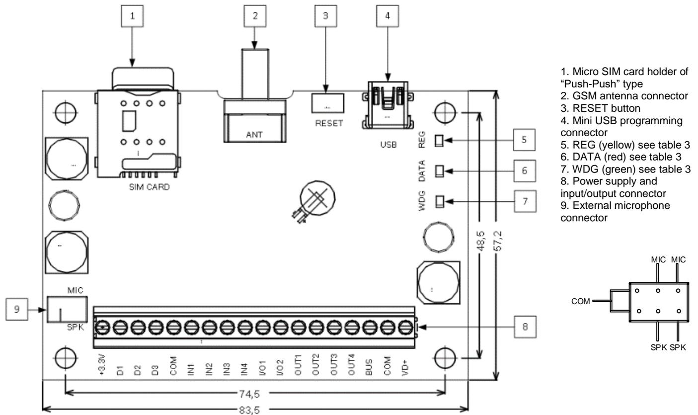
Figure 1 GTalarm2 PCB Layout
