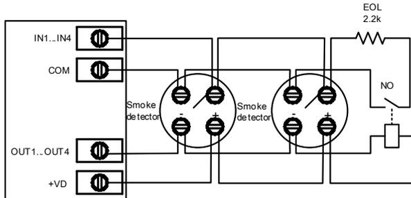
Figure 19 4-Wire Smoke Detector Installation
