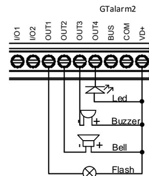
Figure 21 OUT1-OUT4 Open drain 1000 mA connection
