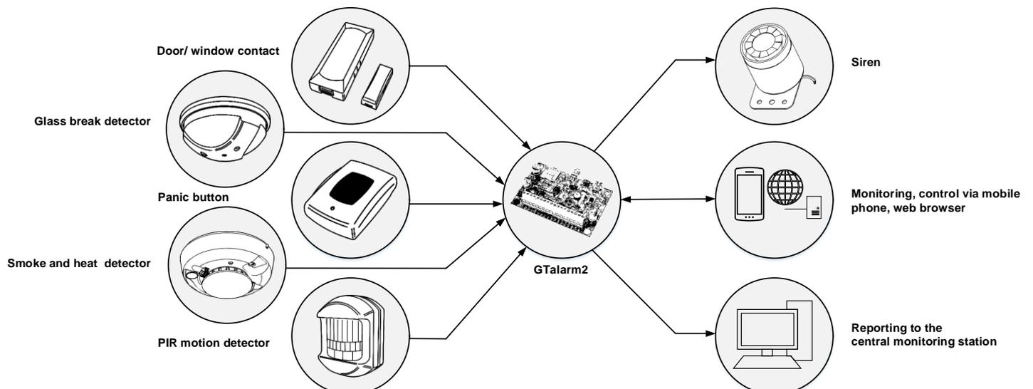
Figure 11 Alarm, remote monitoring, security system
