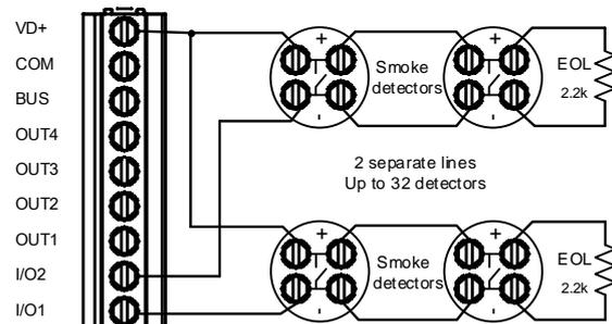
Figure 20 2-wire smoke detector wiring diagram
