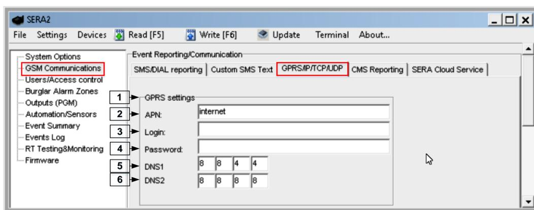
Figure 36 The example of GSM Communication > GPRS/ IP/ TCP/ UDP window
