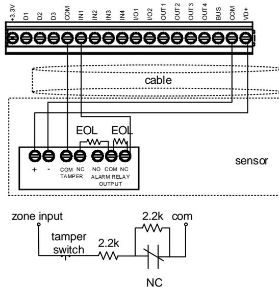
Figure 15 NC With EOL, With Tamper & Wire Fault Recognition
