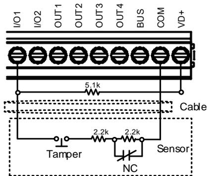
Figure 16 EOL+Tamper sensors connection to I/O1, I/O2
