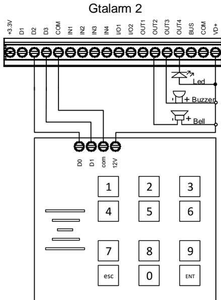
Figure 25 Wiegand keypad connection
