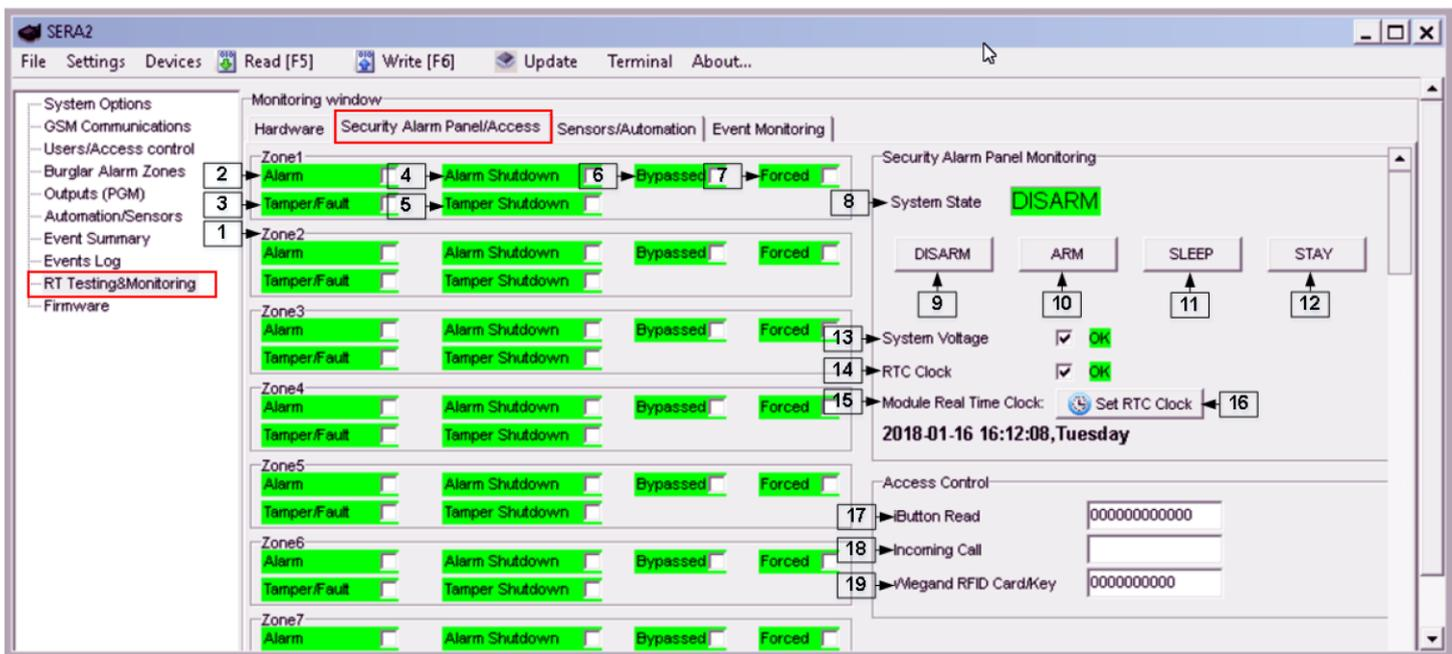
Figure 40 the example of RT Testing & Monitoring > Security Alarm Panel/ Access window
