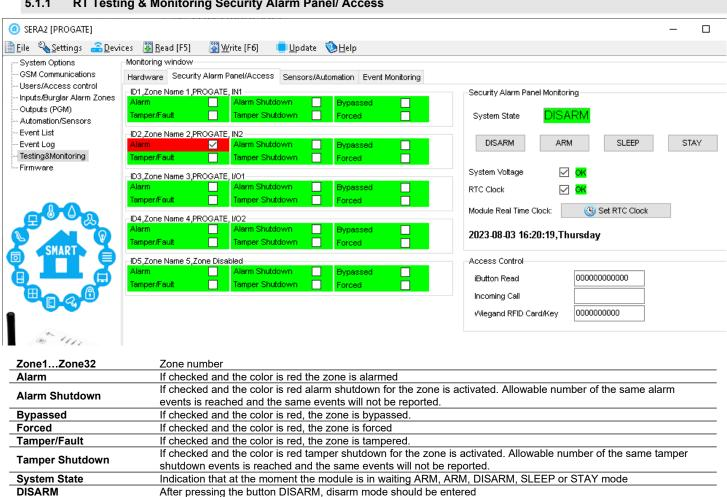
After pressing the button ARM, arm mode should be entered
