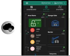
Arming and Disarming the System Using the SERANOVA Mobile/Web App Press on ARM, ARM (Stay), ARM (Sleep), or DISARM in the Mobile/Web App > System window.
